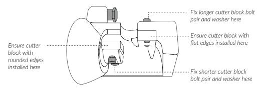
Check cutter block bolts for tightness before each use. Use protective gloves when handling cutter blocks as edges are very sharp.
